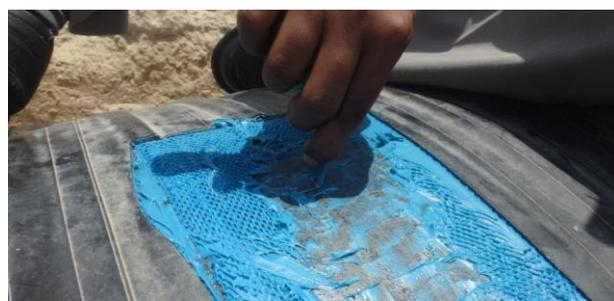
Fig. 3 Peel test: months: a cohesive adhesion and excellent coating condition.
